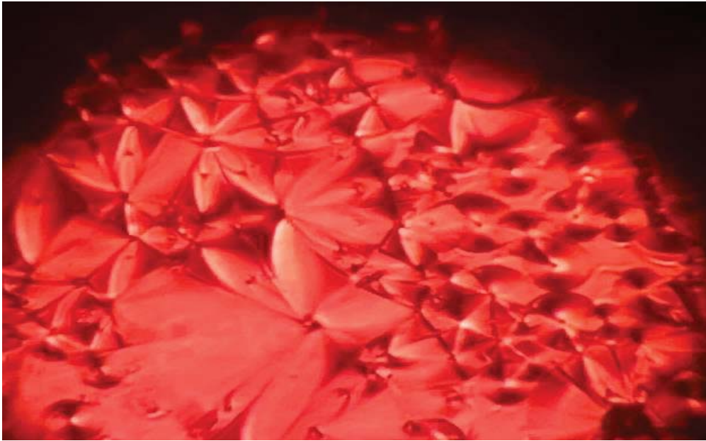
Figure 3: Microphotograph of focal conic texture SmA mesophase(Series I; n=4 ) at 200 °C on cooling
