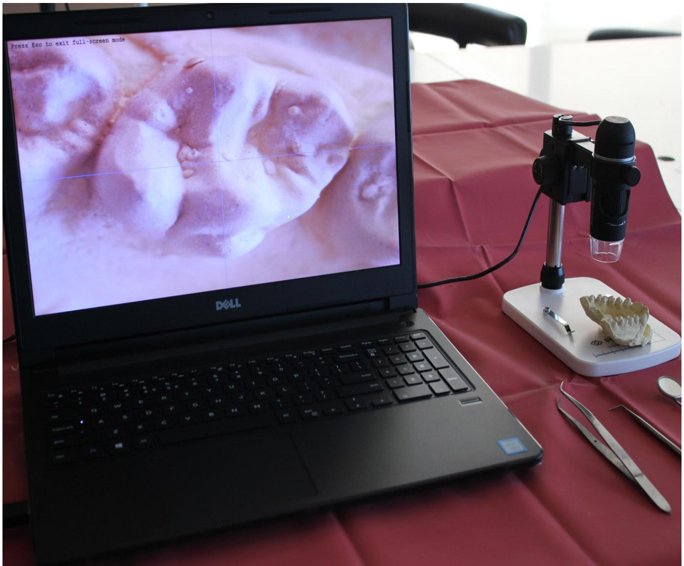
Figure 4 – Picture courtesy from National Forensic Science laboratory showing equipment used for the process such as stereomicroscope for accurate and better vigilance, laptop to be connected with microscope, cast and basic diagnostic tools of Dental.
