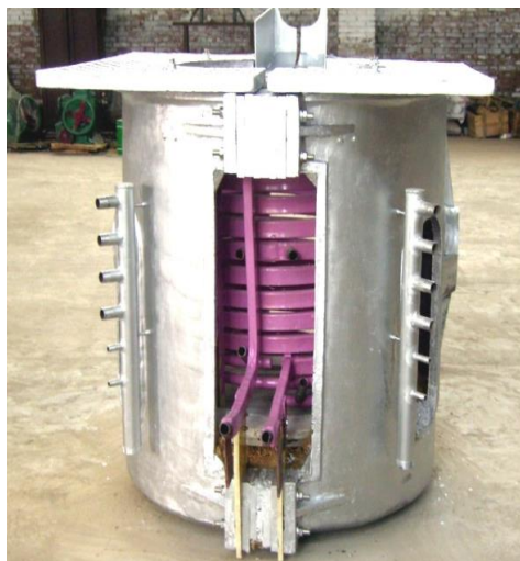
Figure:2 Induction furnace
